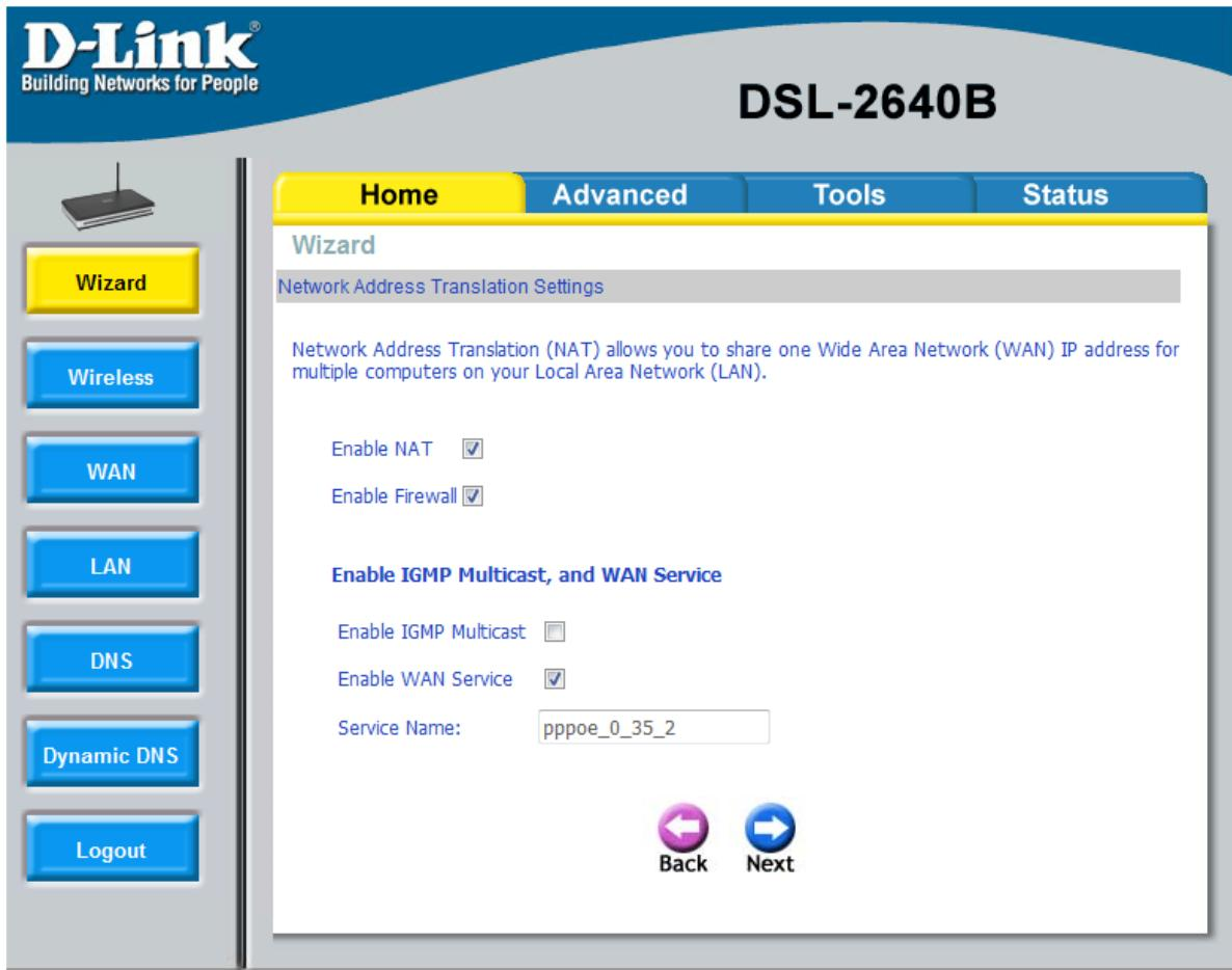
Check “Enable NAT”, “Enable Firewall” and “Enable WAN Service”.
