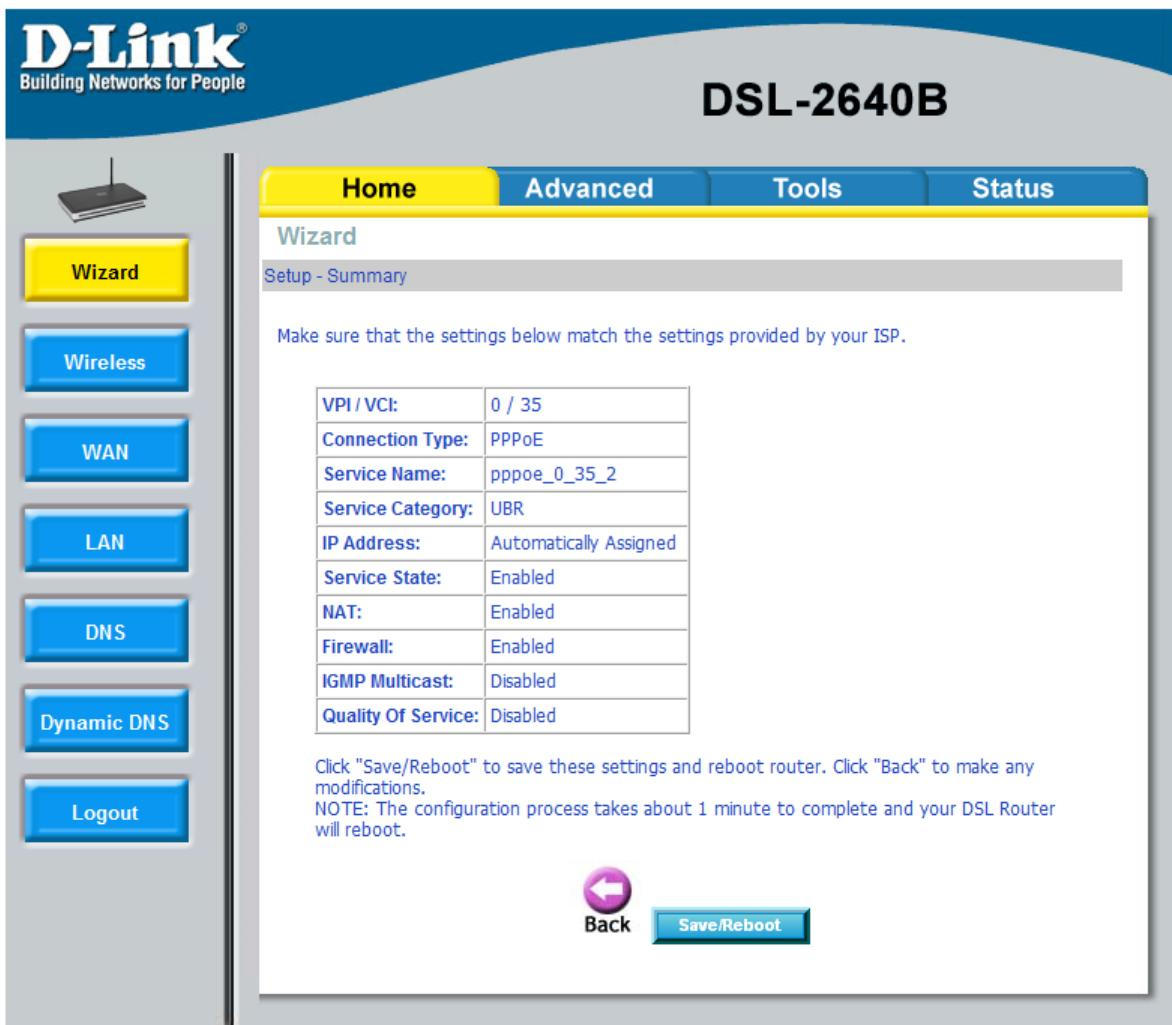
This is the end of the Setup Wizard. Push the "Save and Reboot" button. The modem will now reboot and apply the settings. When the reboot is completed, you can push the "Logout" button, or use one of the other buttons to perform additional setups, as required for your own preferences. Information on the other features of the modem are available in the user manuals for each modem which are included on the Laurel DSL Resources disc and on the support page of the LaurelDSL.net web site.
